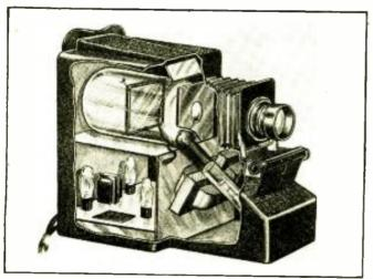
Fig. C. Phantom view, high-fidelity television "camera" shown pictorially in Fig. 8.
